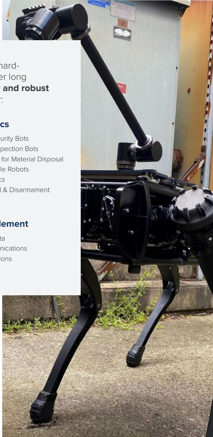
*Pictured here and on first page header, middle image: Ghost Robotics Vision60 version 4 robot with arm by HDT Global. Photos courtesy of Rajant's partner Ghost Robotics.*
